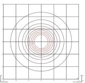
Efficiency Coordinate System Total Flux Maximum Value 46.61 lm/W CG 1842.25 lm 186.24 cd
