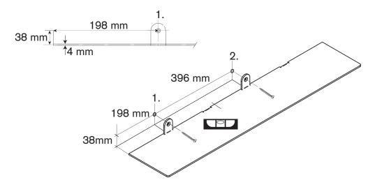
3. - drill the first 2 holes / predrill with Ø 6mm, and drill final hole with Ø 8mm - screw by hand the full coloured wall screws into the connection points! not completely tight to the end!
