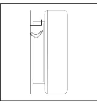
Place the lamp over the L-brackets through the holes provided.
